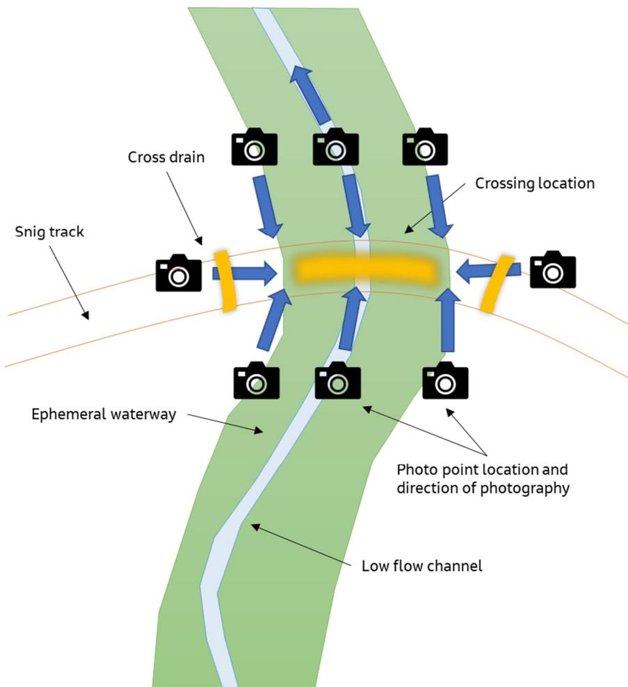
Figure 7-1. Depiction of potential photo point layout for monitoring temporary log crossings
