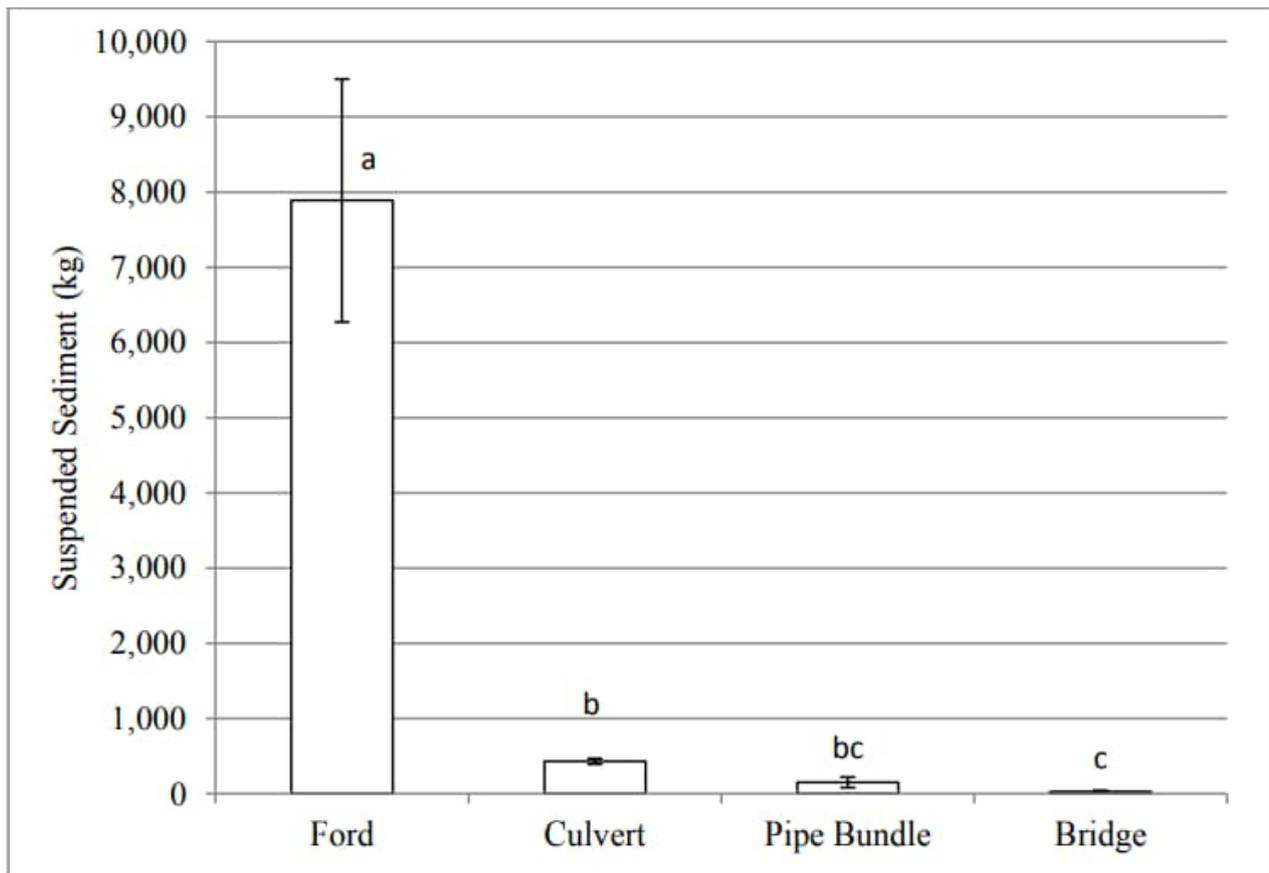
Figure 5-5 Total suspended sediment (mean and standard error) among all crossing types. Different letters indicate significant differences ( $p \leq 0.05$ ) using least squares difference. Source: Reeves (2012)
