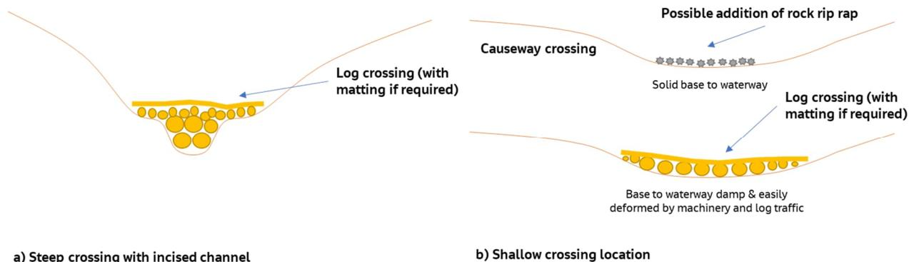
Potential advantages in using temporary log crossings are greater for waterways with steep approaches and/or incised low flow channels. Causeways (with or without rip rap) are suitable for use in settings with lower slope and dry and solid soils that are less likely to be deformed by machinery traffic.
