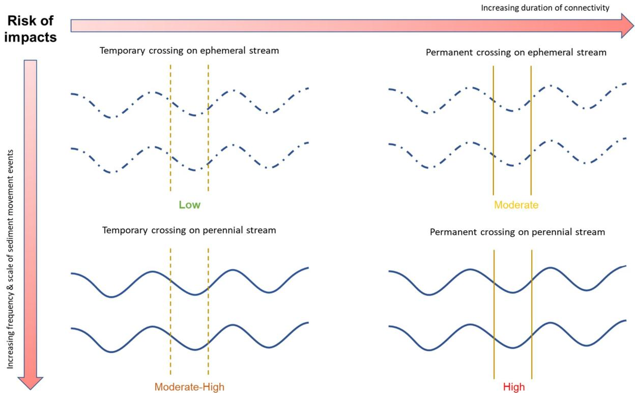
Figure 2-2 Conceptual risk matrix for temporary and permanent track crossings of ephemeral and perennial streams.
