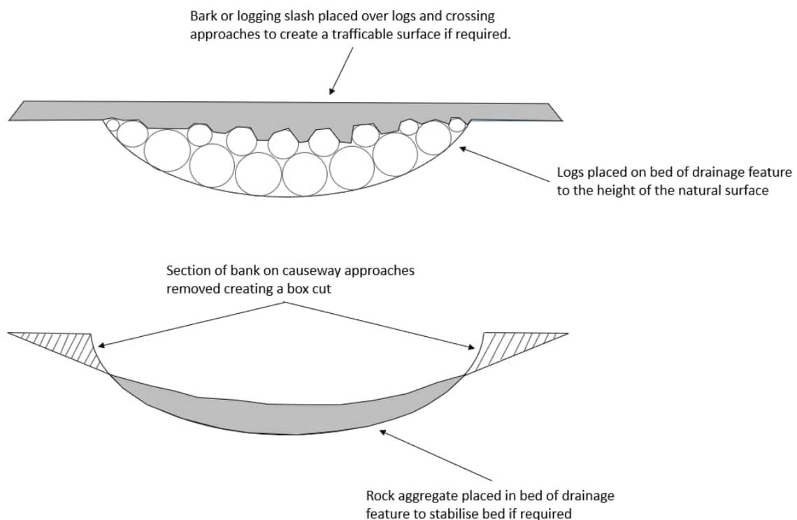
Figure 6-1. Conceptual models of temporary log crossings and causeway crossings for snig tracks (adapted from NSW Forestry Corporation, 2021).
